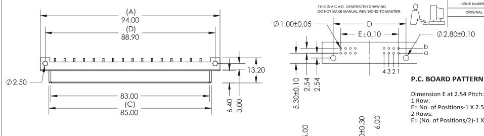
2.90±0.30 10.20 2.54 Dimension E at 2.54 Pitch: E= No. of Positions-1 X 2.54 E= (No. of Positions/2)-1 X 2.54
