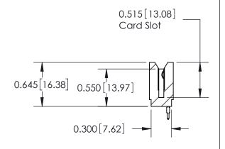
737 Series Ultra-Mate Card Edge Connector - Press Fit Part Number: 737-007-525-106
