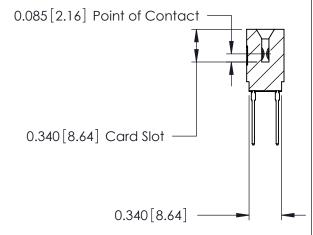
ACAD REFERENCE NO. 746 Series Ultra-Mate Card Edge Connector - Press Fit DRAWN: J.LEE Part Number: 746-010-540-601 CHECKED: **EDAC INC** SCALE: THESE DRAWINGS AND SPECIFICATIONS ARE THE PROPERTY OF EDAC INC.,AND TORONTO, ONTARIO SHALL NOT BE REPRODUCED, OR COPIED DRAWING NUMBER CANADA OR USED AS THE BASIS FOR THE 746-ENG MASTER MANUFACTURE OR SALE OF APPARATUS YOUR CONNECTION TO QUALITY & SERVICE WITHOUT WRITTEN PERMISSION.
