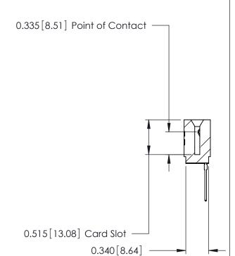
ACAD REFERENCE NO. 746-ENG MASTER 746 Series Ultra-Mate Card Edge Connector - Press Fit DRAWN: J.LEE DATE: AUG 20/09 Part Number: 746-010-545-101 CHECKED: DATE: **EDAC INC** SCALE: SHEET 1 OF 1 THESE DRAWINGS AND SPECIFICATIONS ARE THE PROPERTY OF EDAC INC.,AND TORONTO, ONTARIO SHALL NOT BE REPRODUCED, OR COPIED DRAWING NUMBER **ISSUE** CANADA OR USED AS THE BASIS FOR THE 746-ENG MASTER MANUFACTURE OR SALE OF APPARATUS YOUR CONNECTION TO QUALITY & SERVICE WITHOUT WRITTEN PERMISSION.
