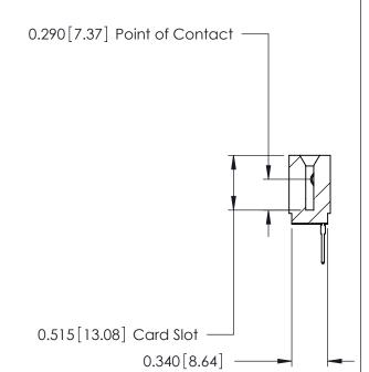
ACAD REFERENCE NO. 746-ENG MASTER 746 Series Ultra-Mate Card Edge Connector - Press Fit DRAWN: DATE: AUG 20/09 J.LEE Part Number: 746-015-527-101 CHECKED: DATE: **EDAC INC** SCALE: SHEET 1 OF 1 THESE DRAWINGS AND SPECIFICATIONS ARE THE PROPERTY OF EDAC INC.,AND TORONTO, ONTARIO SHALL NOT BE REPRODUCED, OR COPIED DRAWING NUMBER CANADA OR USED AS THE BASIS FOR THE 746-ENG MASTER MANUFACTURE OR SALE OF APPARATUS YOUR CONNECTION TO QUALITY & SERVICE WITHOUT WRITTEN PERMISSION.
